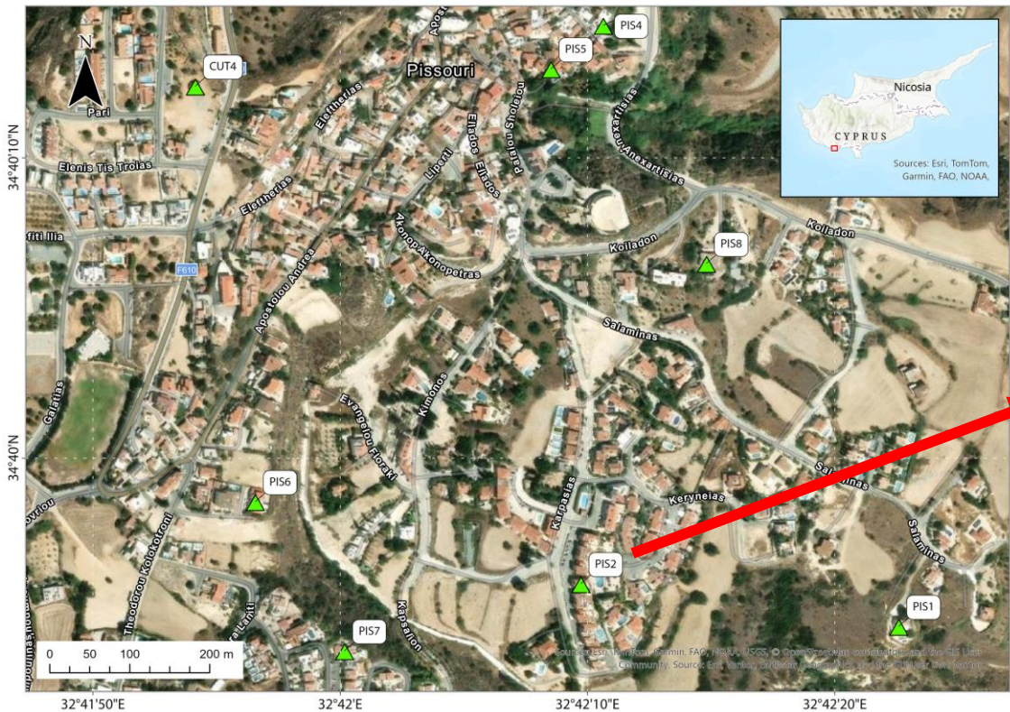
The PIS stations monitor spatially variable ground motion across the affected area.
